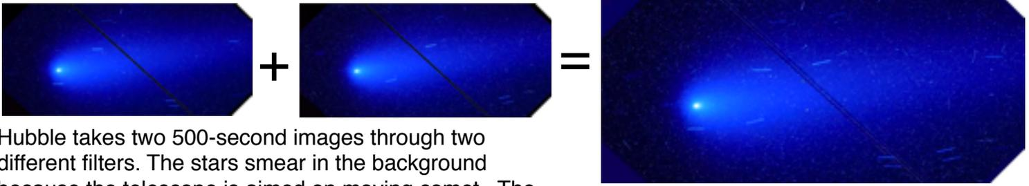
Hubble takes two 500-second images through two different filters. The stars smear in the background because the telescope is aimed on moving comet. The bright speckles, different in each frame, are from random cosmic ray strikes on the detector. The black bar is from the camera's chip. Note the shift of background star trails in the time between exposures.
